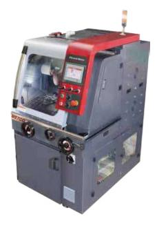
Large heavy-duty cutting machine for sectioning large samples. Has similar features to UM model, but with higher capacity (Z, Y and X movements).
