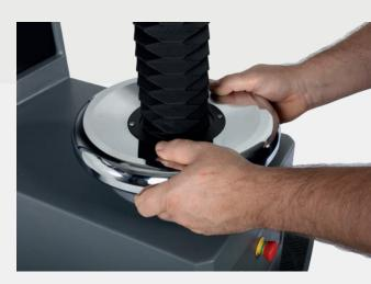
Large handwheel Better grip for simpler clamping of the specimen
